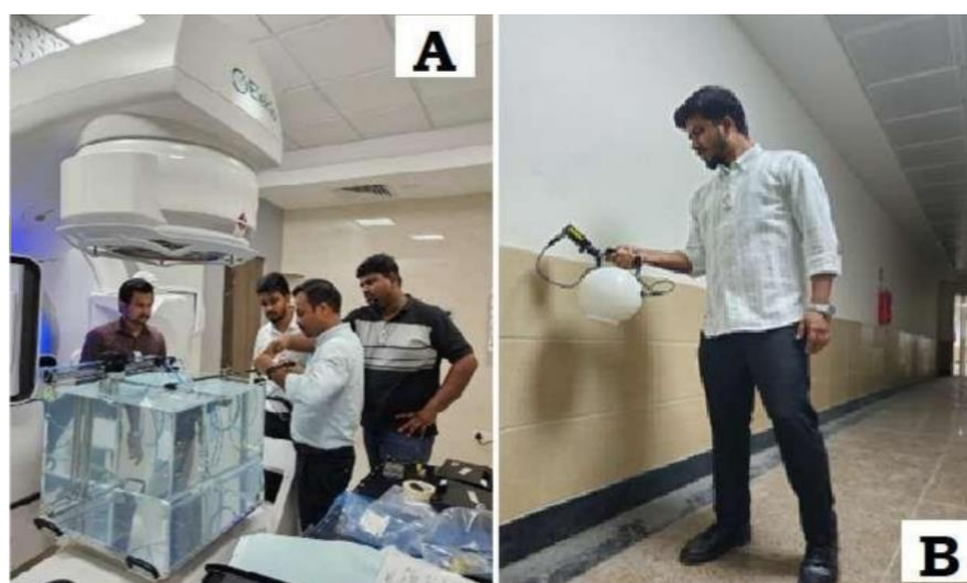
Figure 2: A) Machine-specific QA being conducted by team at Department of Radiation Oncology, AIIMS, Guwahati. B) Radiation protection survey being conducted by an expert in the department with a hand held radiation dosimeter.
